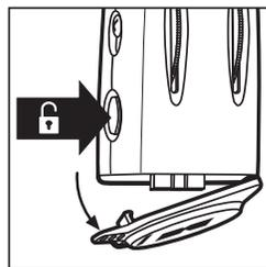
Press the die plate release button to move the die plate away from the date bands
